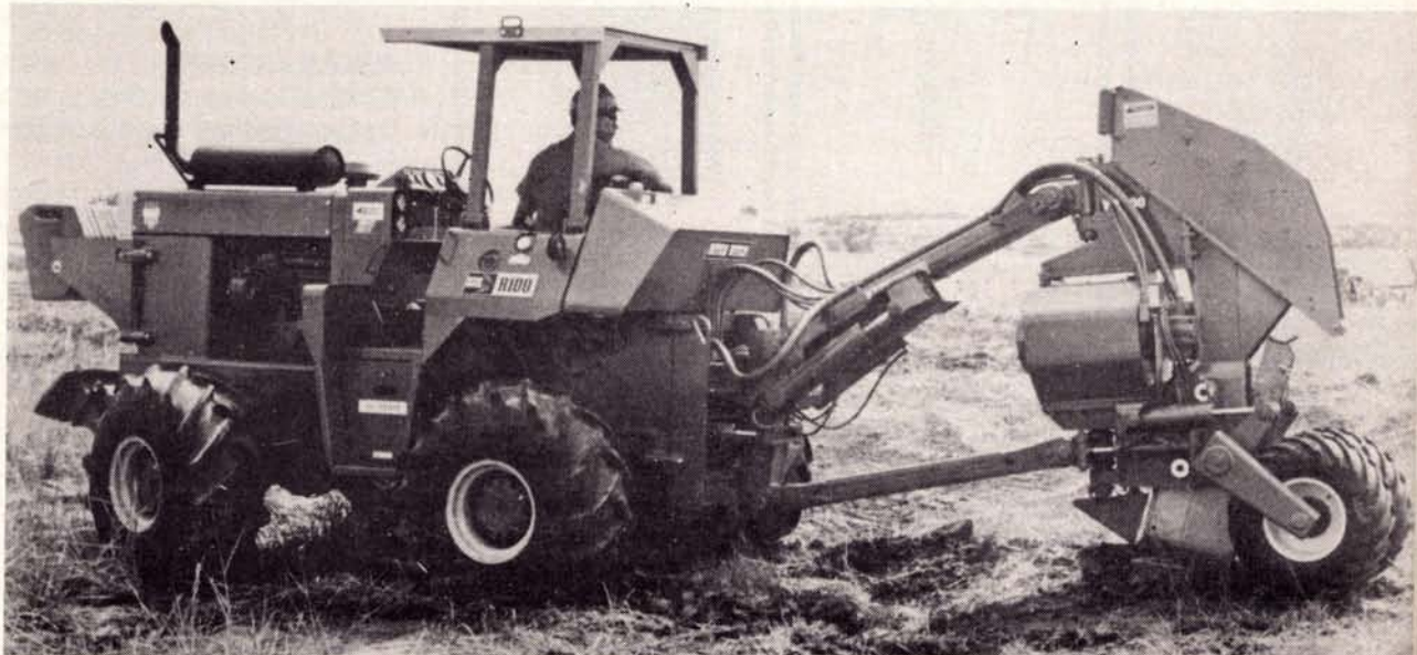
Most powerful in the "Ditch-Witch" series of continuous trenching machines, the Model R100 is shown here with the vibratory plow module.
